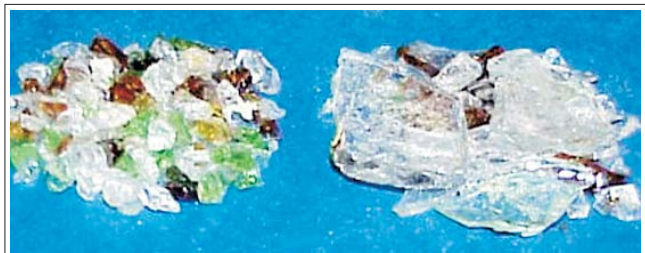
Container glass can be pulverized into different grades of aggregate. The glass on the left has rounded edges and poses no danger to construction workers. The glass on the right was processed with a much less expensive pulverizing machine, resulting in small, sharp shards. Either grade is suitable as fill in road construction and culvert projects.
