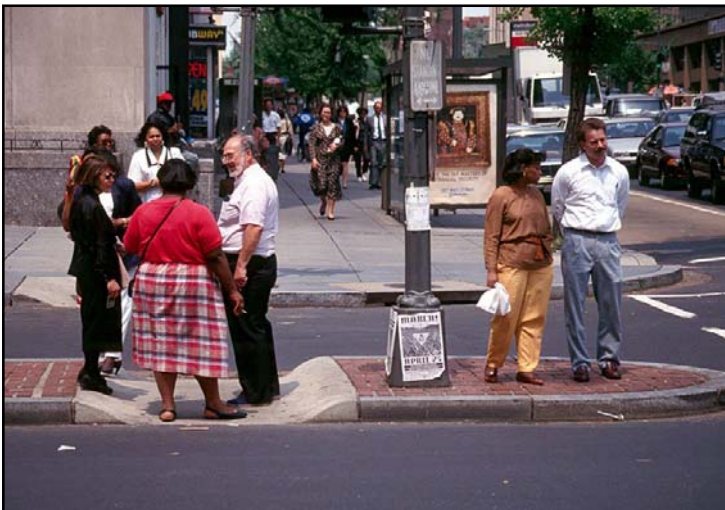
This photo shows pedestrians standing on a depressed median, four-lane separator. It might be safer under certain traffic conditions for the pedestrians to wait for the light to change on the corner of the road.
